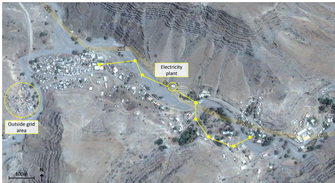
Figure 9 MV distribution line in Randa
